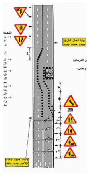
Figure (11-8): An application model - a double road without a middle island in the case that two lanes are closed in one direction.
